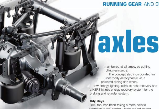
comes as an RSS1360 - a single reduction solo axle, designed for use on high powered trucks up to 60 tonnes.
